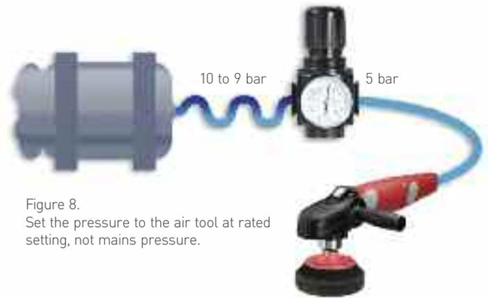
Figure 8. Set the pressure to the air tool at rated setting, not mains pressure.
