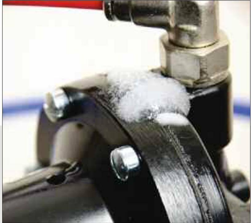
Figure 5. Leakage can be from any joint and is easily shown by spotleak.
