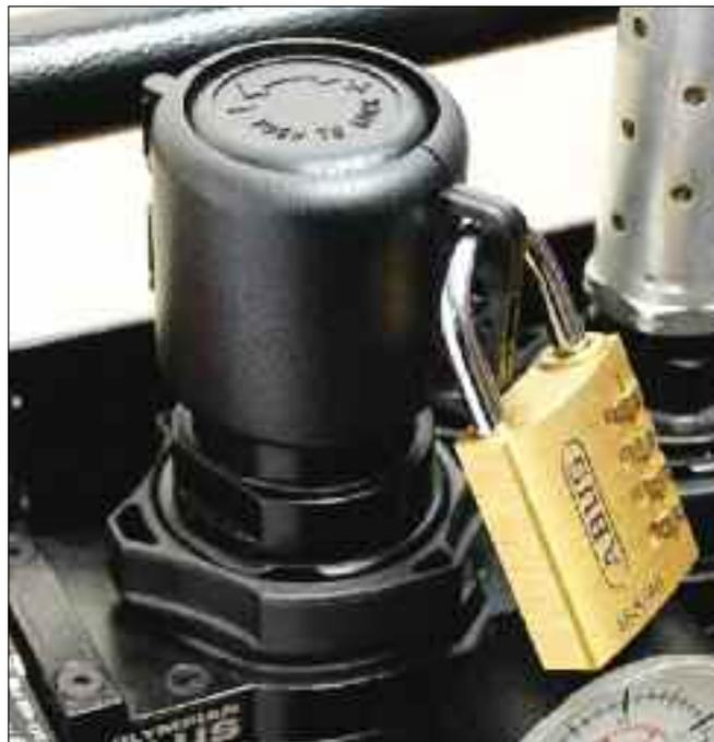
Figure 14. Use of a lockable tamper evident cover on a filter/regulator.
