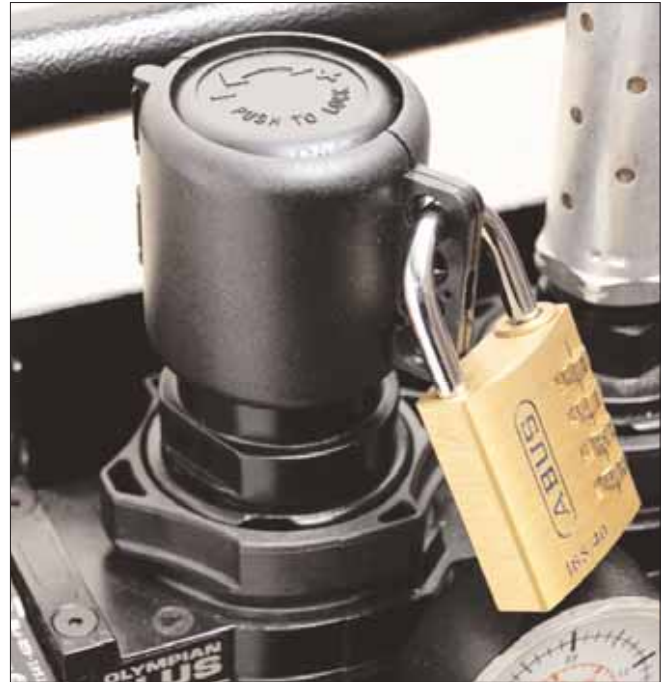
Figure 14. Use of a lockable tamper evident cover on a filter/regulator.
